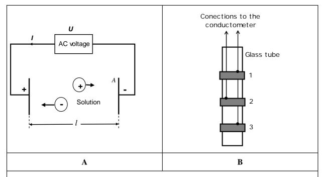
**Fig. 1.** (A) Schematics of conductance measurement setup. (B) The conductometric *probe*  $(pr\phi vesonde)$ . 1, 2, and 3 are platinized platinum sheets; 1 and 3 are electrically connected and form the two parts of a split electrode.
